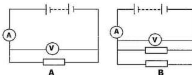
What are the ammeter and voltmeter readings in the circuit shown in 'B' with two resistors?
