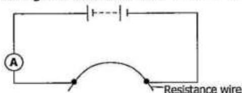
Four separate changes are made to the wire. Which change will **not** reduce the value of the resistance of the wire?
