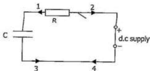
Which arrows show the direction of the conventional current when the capacitor is charging?
