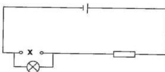
Which component is used as a sensor at **X**?
